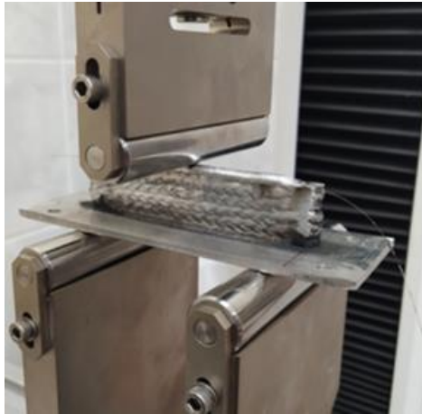
Fig.3. Aluminium component with embedded metal coated optical fiber during 3-point bending tests.
